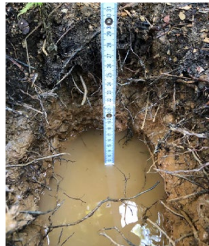
Percolation test for the Woodland Walk Expansion Project.
